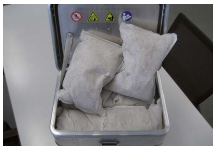
Thermal insulation material, e.g. Vermiculite
